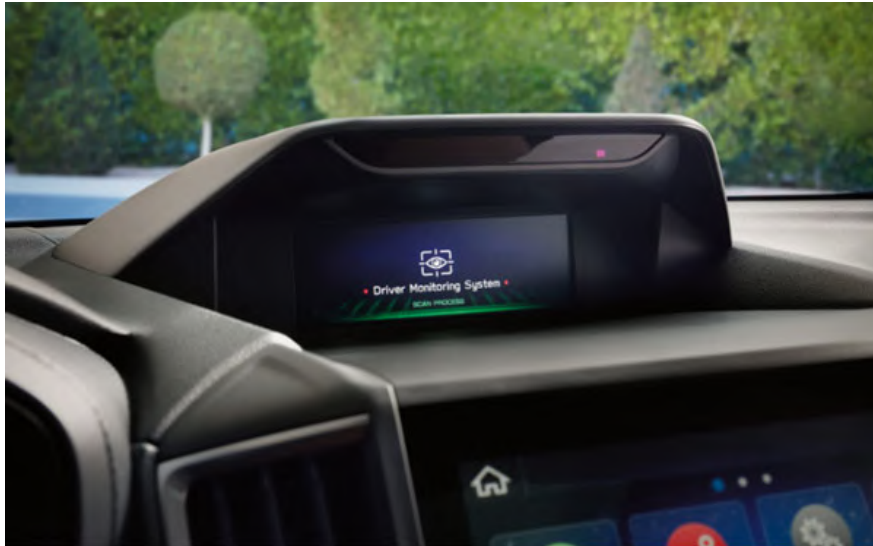
SUBARU DRIVERFOCUS WITH CAMERA AND NIR SOURCE TO TRACK DRIVER GAZE (IMAGE: PLANET SUBARU)
