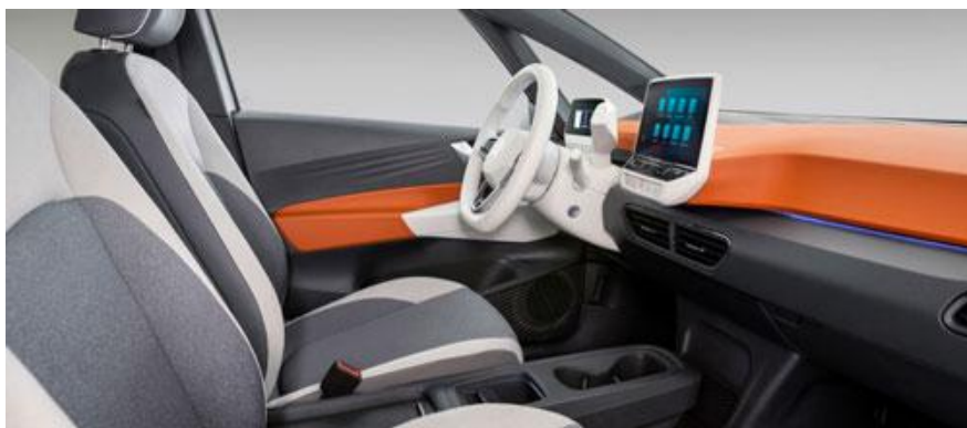
ID.3 cockpit integrates a lighting element between the upper and lower IP.
