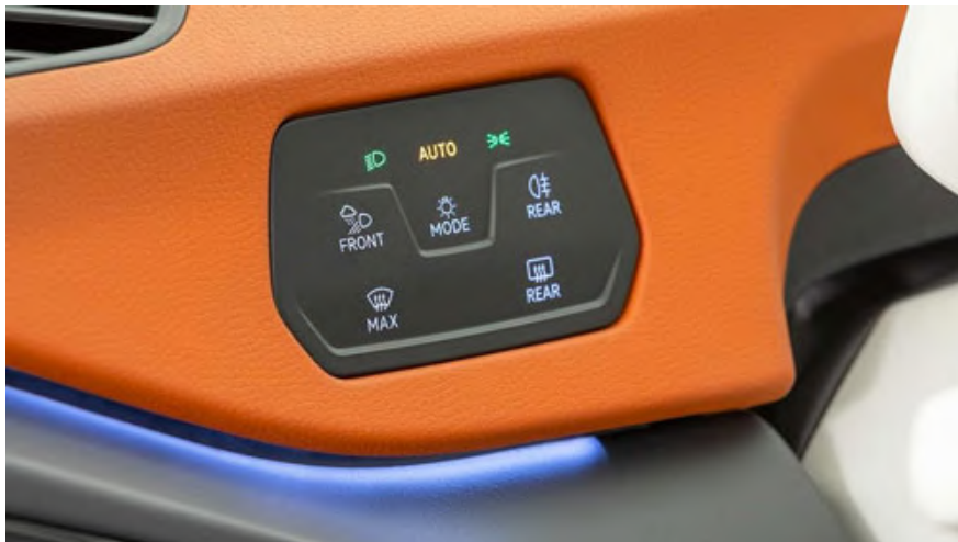
Volkswagen ID.3 capacitive lighting and defogging switch pack
