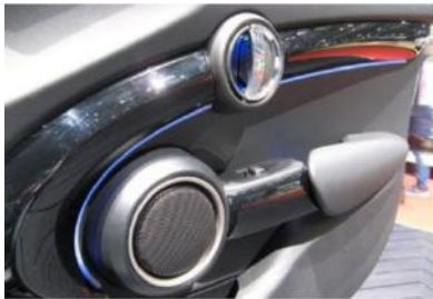
MINI with contour lighting, illuminated door opener, and communication light in combination instrument
