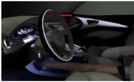
Audi with indirect, contour and smart area lighting in deco trims, cupholders and below center console
