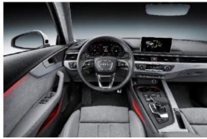
Audi with indirect, contour and smart area lighting in deco trims, cupholders and below center console
