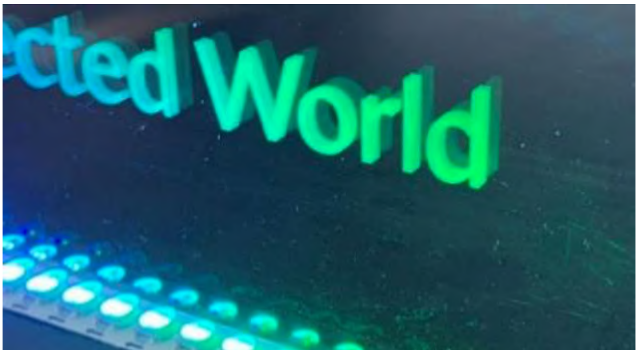
THREE DIMENSIONAL LETTERS, LASERED INTO THE VOLUME OF A LIGHT GUIDE
