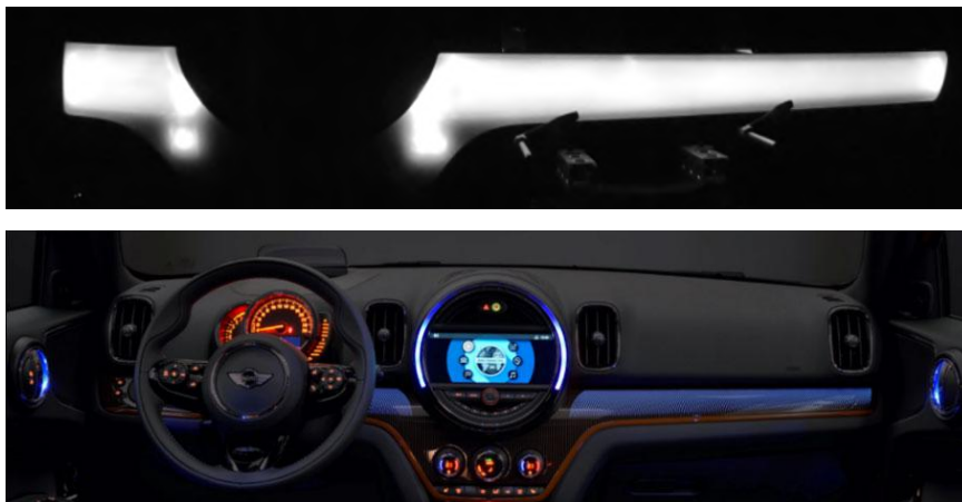
Figure 2: The sill plate has an overall height of < 5\text{mm} with a slim light guide (height 1.5\text{mm} ) and 3 million microstructure elements for a uniform illuminated company logo
