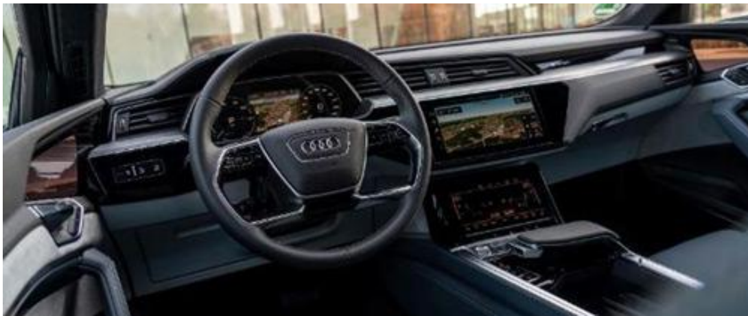
2020 AUDI E-TRON: DISPLAYS (INCLUDING SIDEVIEW CAMERA DISPLAYS) FULLY INTEGRATED INTO THE IP. BUTTONS AND SWITCHES LARGELY DELETED. STRONGER FLOOR/TUNNEL CONSOLE EMPHASIS
