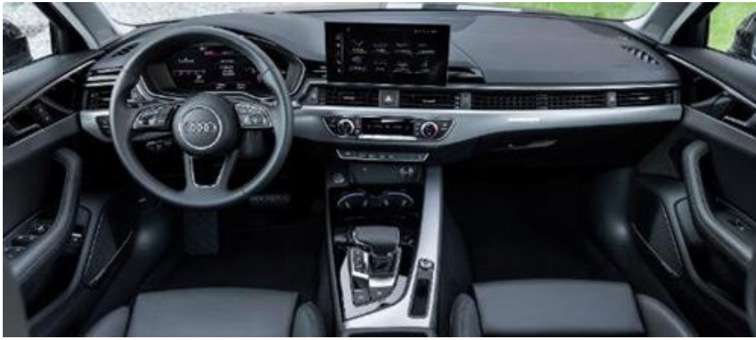
2019 AUDI A4: HORIZONTAL FORM LAYERING WITH SCREENS REPLACING THE CLUSTER AND A TABLET TYPE FLOATING DISPLAY
