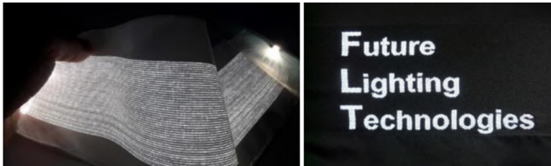
SOURCE FA.FLT: TEXTILES WITH WEAVED LIGHT GUIDING THREADS
