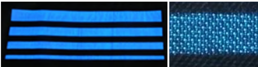
SOURCE FA.FLT: LIGHTED TEXTILES WITH PRINTED ELECTROLUMINESCENCE PASTE
