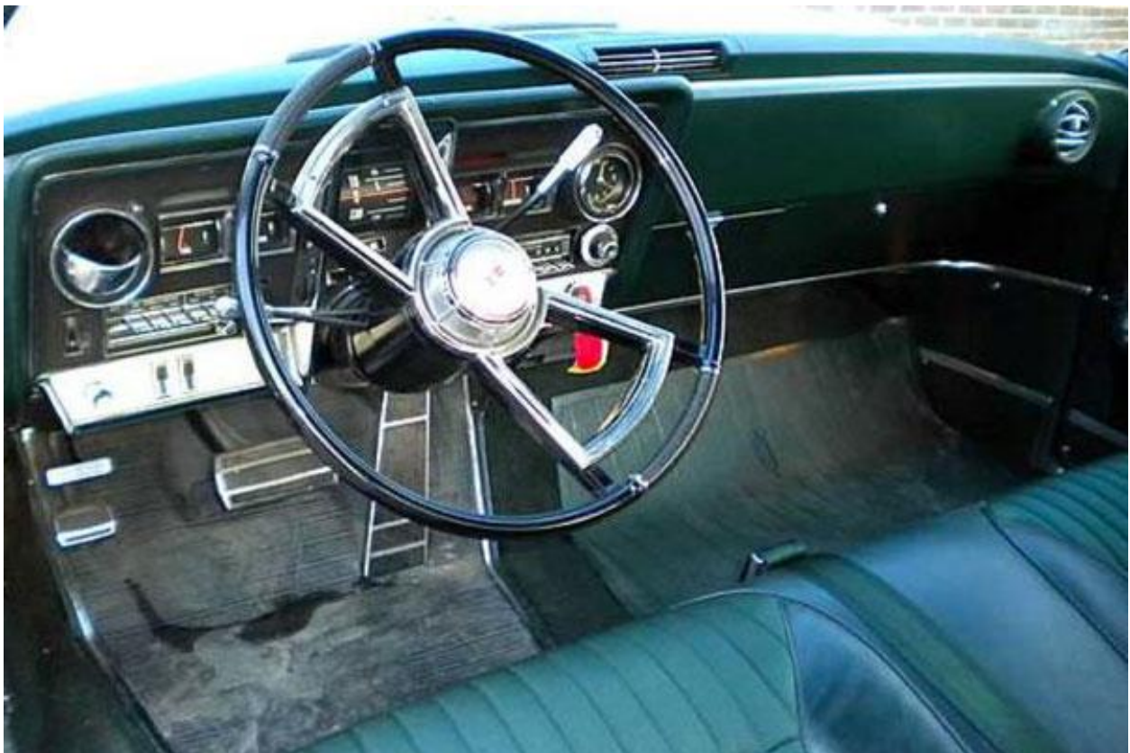
1967 OLDSMOBILE TORONADO WITH A COLUMN SHIFT AND A TUNNEL FREE FLOOR ENABLED BY ITS FRONT WHEEL DRIVE
