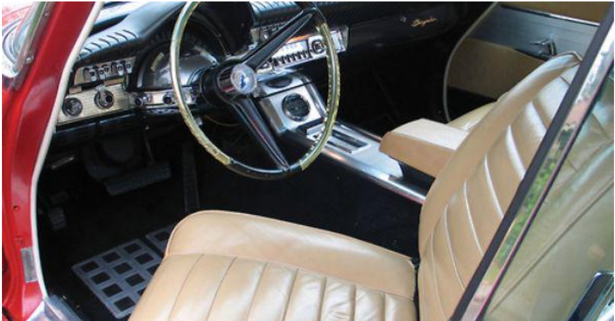
1961 CHRYSLER 300 WITH A PUSHBUTTON TRANSMISSION AND A FULL LENGTH CENTER CONSOLE (YES, THOSE ARE ALSO SWIVEL SEATS)
