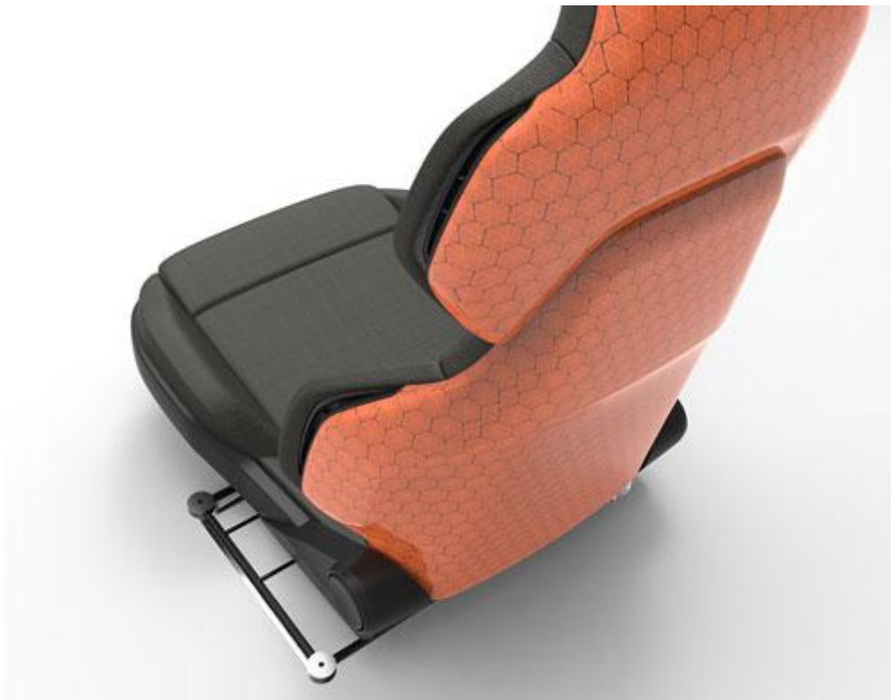
ULBS with a back panel shell made of intralaminar reinforcing core (IRC) material, and 3D-printed seat backrest cushions made from thermoplastic polyurethane (TPU).
