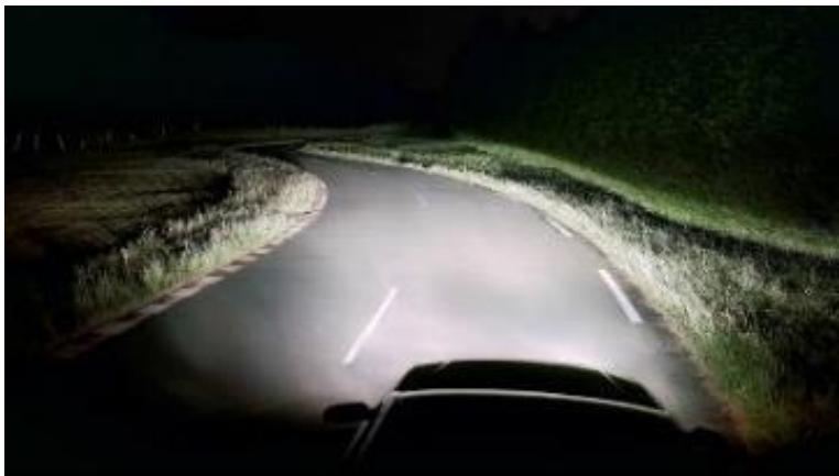
HID headlamp with bending light
