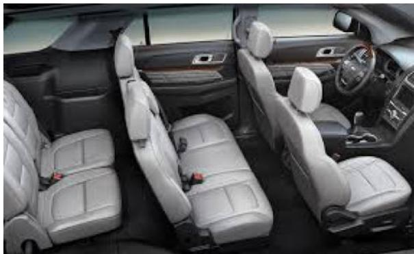
Ford's global seating and design team has maintained the comfort standard in the new Explorer's front-row seat while eliminating some of the bulk by reducing the thickness of the seatback and shoulder area. The main target of a less-cumbersome front seat design is to maintain the same comfort standard (especially torso support) while freeing up space for second-row passengers.
