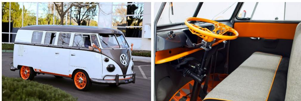
The Type 20 concept uses the body of a 1962 Type 2 Microbus as its base, but the underpowered, gross-polluter gasoline engine and powertrain have been replaced with a 120-hp electric motor and small 10-kilowatt-hour battery with a 2,500-watt onboard charger. A pneumatic suspension system was borrowed from Porsche to adjust the vehicle's ride height via software, including when the driver approaches the vehicle.
