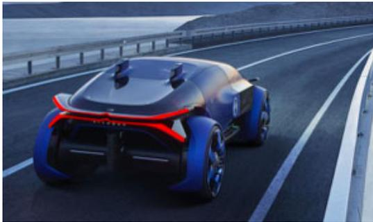
Dual lidar sensors mounted at the rooftop complement the array of sensors enabling the vehicle to drive autonomously; besides the lidars, they include radar and camera sensors.
